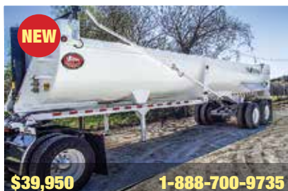
NEW $39,950 1-888-700-9735 2018 CTS Rockmaster HRD AR 450 End Dump, 32' x 102", Spring Suspension, 11R24.5 Tires, Electric Tarp. New . (JS000099-WAC-3)
