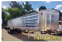
2017 Travis Wave 39 Ft. Aluminum End Dump, Air Ride, Lift Axle, Roll Tarp, Liner, 11R24.5 Tires, All Aluminum Floor. New. (H1011613-TYL-TRL-2b)
