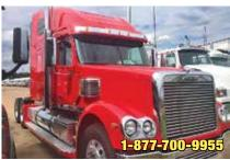
2016 Freightliner Glider, Detroit Series 60 12.7 Engine Pre-Emissions, 500 HP, 13 Spd, 3.55 Ratio, 260" Wheelbase, 11R22.5 Tires, All Aluminum Wheels. New Glider. (DGGS5401-SHV-1)
