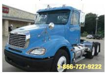
2009 Freightliner Columbia 120, SER 60 14.0L 455 hp; Diesel; 10 Spd; Air Ride Suspension; 3.58 Ratio; 22.5 LP Tires; Aluminum Wheels; 176 in Wheelbase. (9LAG2423-BRY-2)
