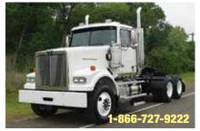
2014 Western Star 4900, DD15 Detroit Engine 505 hp; Diesel; 10 Spd; Air Ride Suspension; 3.73 Ratio; 24.5 Tires; All Steel Wheels; 215 in Wheelbase; Tandem Axle; 14,700 lb Front Axle Weight; 46,000 lb Rear Axle Weight; 1,500 Miles. (EPFM9894-BRY-2)
