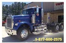
2007 Freightliner FLD12064SD, SER 60 14L Detroit Engine 515 hp; Diesel; 10 Spd OD; Engine Brake; Air Ride Suspension; 3.90 Ratio; 24.5 Tires; Aluminum Outside Wheels; 220 in Wheelbase, 347,915 Miles. (DY62468-TYL-3)
