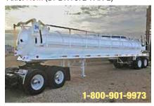
2013 Majona 130 Barrel Vac Tank Trailer, (Qty: 65) 4 Spring Susp; 40 ft Long x 102 in Wide x 1 ft Height; 11Rx24.5 Tires; All Steel Wheels; Fixed Tandem Ax; Steel Comp; Semi Tank; Qty. disc. avail. 130 BBL Steel Vacuum Trailer. New. (DA906181-SAN-TRL-3)
