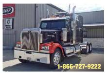
2007 Western Star 4900 EX, Mid Roof Sleeper; SERIES 60 14L Detroit Engine 515 hp; Diesel; 10 Spd; Air Ride Suspension; 3.73 Ratio; 24.5 Tires; Aluminum Wheels; 265 in Wheelbase, 601,500 Miles. (7PY17114-BRY-3)
