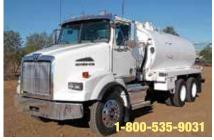
2012 Western Star 4900 Vacuum Tank Truck, (Qty: 2) DD13 Detroit 450 hp; Diesel; 8LL; Eng. Brake; TufTrac Susp; 4.30 Ratio; Aluminum/Steel Wheels; 227 in WB; Tandem Axle; 24.5 Tires; 46,000 lb Rear Axle Weight; 14,600 lb Front Axle. New. (CPBM8294-FAR-1)
