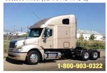
2007 Freightliner Columbia, 70" Raised Roof Sleeper, Detroit Series 30 14L, 10 Spd, Air Ride Suspension, 3.58 Ratio, 22.5 LP Tires, All Aluminum Wheels, 783,500 Miles. (7LW40409-WFF-3)
