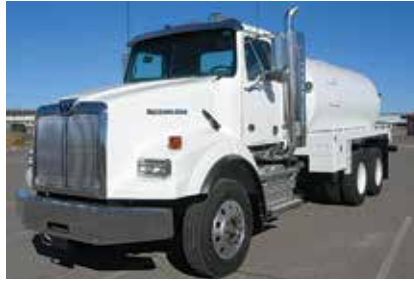
2012 Western Star 4964SA Vacuum Tank Truck, ISX Cummins Engine 485 hp; Diesel; 8LL; Engine Brake; TufTrac Suspension; 4.30 Ratio; Aluminum/Steel Wheels; 227" WB; Tandem Axle; 24.5 Tires. New. (CPBK9610-FAR-3)
