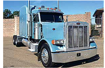
2003 Peterbilt 379EXHD, 63 in Ultracab Unibilt; C15 Caterpillar Engine 475 hp; Diesel; 10 Spd OD; Engine Brake; Air Ride Suspension; 3.55 Ratio; 22.5 Tires; All Aluminum Wheels; Tandem Axle, 919,974 Miles. (3D529424-TYL-3)
