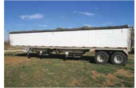
1991 Wilson Grain Hopper, Spring Suspension; 42 ft Length x 96 in Width; Aluminum Floor; 24.5 Tires; Aluminum Wheels; Fixed Tandem Axle; Stainless Steel Composition; 42x96 Wilson Grain trailer. 66" sides, and vibrators. (MA215391-TEX-TRL-3c) $19,500
