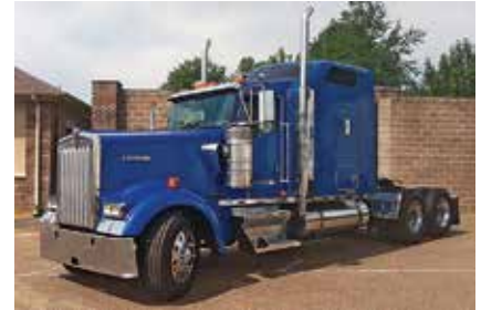
2005 Kenworth W900L, 72 in Aerocab Aerodyne Sleeper; C15 Caterpillar Engine 475 hp; Diesel; 13 Spd OD; Engine Brake; Air Ride Suspension; 3.36 Ratio; 24.5 Tires; Aluminum Outside Wheels; Tandem Axle. (5J085165-TXK-2)
