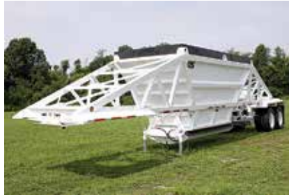
2013 MANAC Light Weight Belly Dump, (Qty: 2) Spring Suspension; 40 ft Length x 102 in Width; Frame; 24.5 Tires; Steel Disc Wheels; Fixed Tandem Axle; Steel Composition; Spring ride, steel wheels, and tarp. (D3139239-TYL-TRL-2b)
