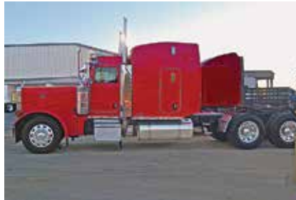
2005 Peterbilt 379EXHD, 63 in Ultracab Unibilt; C15 Caterpillar Engine 475 hp; Diesel; 13 Spd OD; Engine Brake; Air Ride Suspension; 24.5 LP Tires; Aluminum Wheels; 265 in Wheelbase; Tandem Axle, 642,500 Miles. (6D862367-TYL-2)
