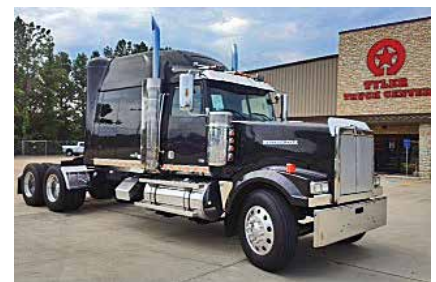
2010 Western Star 4900 EX . Detroit DD15 - 500-560 HP, 13 Spd, 60" Mid Roof Sleeper, Air Ride Suspension, 3.36 Ratio, 265" Wheelbase, 159,382 Miles. (APAV2882-TYL-3)
