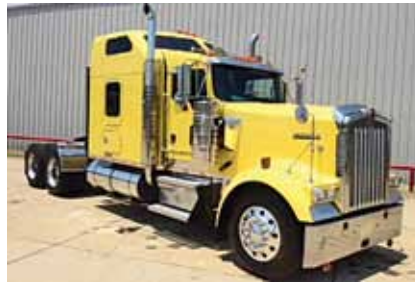
2006 Kenworth W900L , 72 in Aerocab Aerodyne Sleeper; C15 Caterpillar Engine 475 hp; Diesel; 13 Spd OD; Engine Brake; 8 Bag Air Ride; 3.36 Ratio; 11 X 24.5 Tires; All Aluminum Wheels; 266 in Wheelbase; Tandem Axle. (6J112429-SHV-2)
