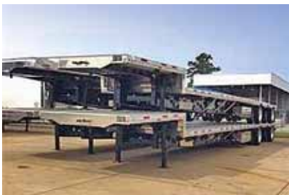
2013 Transcraft Combo Drop Deck, (Qty: 3) Air Ride; 53 ft Long x 102 in Wide; Alum. Floor; 22.5 Tires; Alum. Outside Wheels; Sliding Spread Tandem Axle; Combination Comp; Fixed Neck. New . (D3742652-SHV-TRL-2B) $Call for Price.
