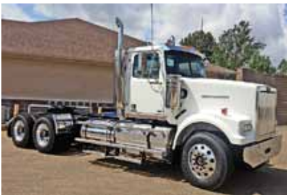
2013 Western Star 4900, Detroit DD15, 505 HP, 10 Spd, 3.90 Ratio, Engine Brake, Air Ride Suspension, 230" Wheelbase, 24.5 Tires, All Aluminum Wheels, 5 Year/500K Engine Warranty. New (DPBW5387-TXK-3)
