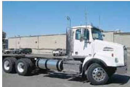
2012 Western Star 4900, (Qty: 2) Standard Cab; DD13 Detroit Engine 450 hp; Diesel; 8LL; Engine Brake; TufTrac; 4.30 Ratio; 24.5 Tires; Aluminum/Steel Wheels; 227 in Wheelbase; Tandem Axle, New (CPBM2894-FAR-3)
