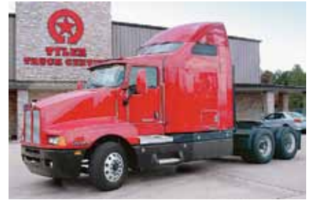
2007 Kenworth T600 , 72 in Aerocab Aerodyne Sleeper; ISX Cummins Engine 450 hp; Diesel; Automatic OD; Engine Brake; Air Ride; 3.36 Ratio; 22.5 LP Tires; All Aluminum Wheels; 240 in Wheelbase. (7J189869-SHV-1) $49,700 $43,500
