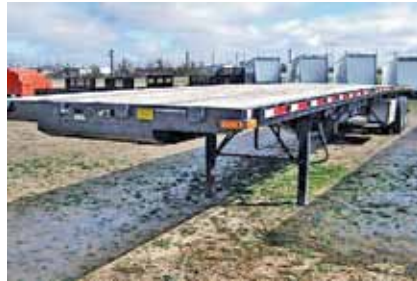
2008 Transcraft Flat Bed , 53' x 102", Air Ride Suspension, Tandem Axle, 11R24.5 Tires, Steel Wheels, Hardwood Floors. (81084591-SAN-TRL-1) $18,500
