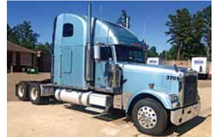
2006 Freightliner FLD132 Classic XL , 70" Sleeper, Caterpillar C15, 9 Spd, 3.58 Ratio, 260" Wheelbase. (6DU25708-TXK-2) $42,500
