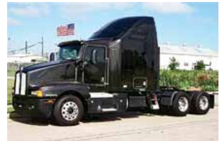
2006 Kenworth T660 , 72 in Premium High Roof; Caterpillar Engine 435 hp; Diesel; 13 Spd OD; Engine Brake; Air Ride; 3.58 Ratio; 22.5LP Tires; Aluminum Outside Wheels; 235" WB; Tandem Axle; 680,000 Miles. (6J109047-WFF-2)
