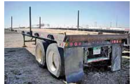
1984 Lufkin Oil Field Float, Spring Susp; 37 ft Long x 96 in Wide; Wood Floor; 24.5 Tires; Steel Disc Wheels; Fixed Tandem Axle; Steel Comp; Hard to Fine Used Oil Field Float With Rolling Tail Board. (E1064496-SAN-TRL-2)
