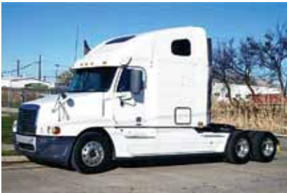
2007 Freightliner CST12064 Century 120 , 70 in Raised Roof Condo; Diesel Detroit Engine 455 hp; 10 Spd OD; Engine Brake; Air Ride; 3.58 Ratio; 22.5LP Tires; All Aluminum Wheels; 236" WB; Tandem Axle; 598,000 Miles. (7LX03451-WFF-3)
