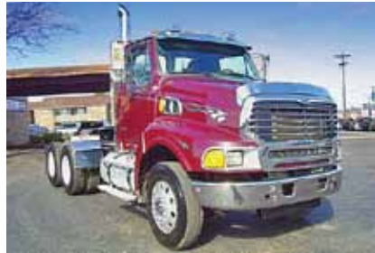
2009 Sterling L9500, DD15 Detroit 560 hp; ; Diesel Fuel Type; 18 Spd OD; Eng Brake; Air Ride; 4.10 Ratio; 24.5 Tires; Alum Wheels; 196 in WB; 14,000 lb Front Axle Wt; 46,000 lb Rear Axle Wt, 233,000 Mileage. (9AAB0130-ABL-3) $67,500
