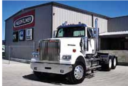
2012 Western Star 4900FA , ISX Cummins Engine 450 hp; Diesel; 10 Spd OD; Engine Brake; Air Ride Suspension; 3.70 Ratio; 11R 24.5 Tires; Aluminum/Steel Wheels; 215 in Wheelbase; Tandem Axle. New. (CDBW8000-TEM-3)
