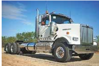
2012 Western Star 4900FA , 275 in WB, DD15 Detroit 560 hp, 18 Spd OD, Jakes, 20K Front, 4.10 Ratio, Neway 52,000 lb Air Ride, 48" A/S 5th Wheel, Dual 125 Gal Alum Tanks, Alum Wheels, Tinted Sliding Rear Window. New. (CPBM7234-SAN-1) Call For Price
