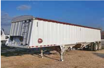
2010 Construction Trailer Hopper Bottom , Leaf Springs Suspension; 40 ft Length x 96 in Width; 11R 24.5 Tires; All Steel Wheels; Fixed Tandem Axle; Steel Composition; 2 Hoppers; Better than New. (AS000538-TEM-TRL-1) $24,000
