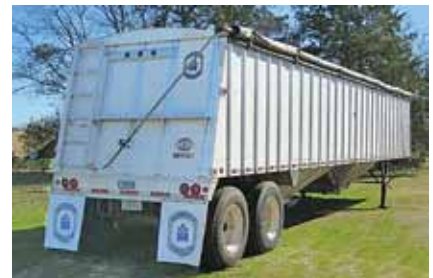
2003 Merritt Hopper Grain Hopper , Air Ride Suspension; 42 ft Length x 96 in Width; Aluminum Floor; 22.5 Tires; Fixed Tandem Axle; Aluminum Composition; 2 Hoppers; Aluminum Air ride Hopper bottom with Rollover Tarp. (3H014476-SHV-TRL-1A) $19,500
