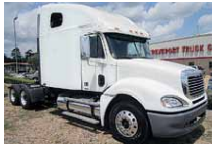
2007 Freightliner Columbia CL120 , 70" Sleeper, Detroit Diesel DDC 14.0, 455 HP, 10 Spd, Air Ride Suspension, 3.58 Ratio, 230" WB, 22.5 LP Tires, All Aluminum Wheels, 498,210 Miles. (7LY88971-SHV-2) $42,500 $39,700
