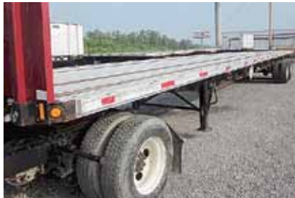
2000 Fontaine Combo Flatbed , (Qty: 2) Spring Susp; 48 ft Long x 102 in Wide; Alum. Floor; 22.5 Tires; All Steel Wheels; Sliding Tandem Axle; Combination Composition; Alum. Combo Spring Slider. 22.5 Tires. (Y5990931-SHV-TRL-3b)
