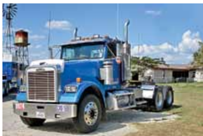
2000 Freightliner FLD120 , Detroit Diesel DDC 12.7, 500 HP, 10 Spd, Air Ride Suspension, 4.33 Ratio, 220" Wheelbase, 24.5 Tires, All Aluminum Wheels, 834,320 Miles. (YPA723331-TYL-2) $23,500
