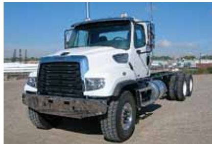
2012 Freightliner 114SD , Standard Cab; DD13 Detroit Engine 450 hp; Diesel; 18 Spd; Engine Brake; TuffTrac Susp; 4.30 Ratio; 24.5 Tires; Alum/Steel Wheels; 260 in WB; 14,600 lb Front Axle Wt; 46,000 lb Rear Axle Wt. (CDBK3308-FAR-3)
