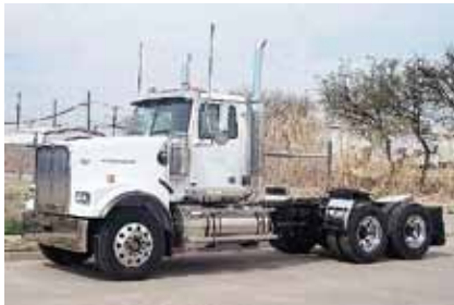
2012 Western Star 4900FA , (Qty: 3) DD15 Detroit Engine 505 hp; Diesel; 10 Spd OD; Engine Brake; Air Ride Suspension; 3.70 Ratio; 11R24.5 Tires; All Aluminum Wheels; 220 in Wheelbase; Tandem Axle, (CPBL2636-WFF-3) New .
