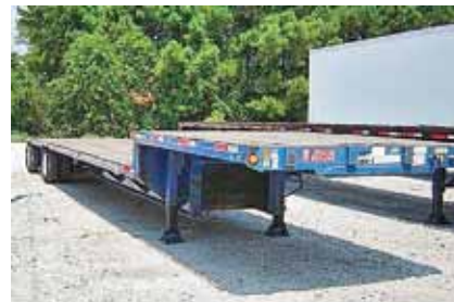
2000 Fontaine Drop Deck , (Qty: 6) Air Ride; 48 ft Long / 102 in Dide; Apitong Floor; 22.5 Tires; Steel Disc Wheels; Spread Tandem Ax; Steel Comp.; Wide Spread Air ride, Container locks 1-20' container. Trailer has 11' upper deck / 37' bottom deck. (Y5993422-SHV-TRL-1A) Call for Price
