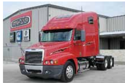
2008 Freightliner CL12064ST Century 120 , 70 in Raised Roof Condo; 14.0 Detroit Engine 500 hp; Diesel; 10 Spd OD; Engine Brake; Air Ride Suspension; 3.42 Ratio; LP 22.5 Tires; All Aluminum Wheels; 230 in Wheelbase; Tandem Axle, 559,150 Miles. (8LAB3328-BRY-1) $59,750
