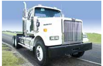
2012 Western Star 4900 FA Day Cab, Detroit Diesel DD15, 475 HP, 10 Spd, Air Ride Suspension, 3.73 Ratio, 215" Wheelbase, 24.5 Tires, Steel Wheels Front & Back, New. (CPBJ3904-BRY-3)
