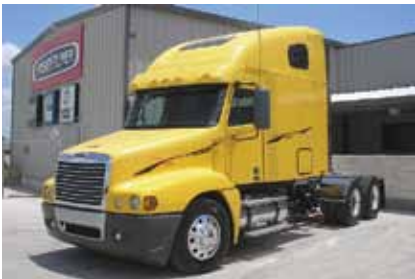
2008 Freightliner CL12064ST Century 120, 70 in RR Condo; 14.0 Detroit 500 hp; Diesel; 10 Spd OD; Engine Brake; Air Ride; 3.42 Ratio; LP 22.5 Tires; All Aluminum Wheels; 230" WB; Tandem Axle. 475,000 Miles. (8LAB3321-WAC-2)
