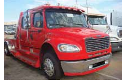
2007 Freightliner RHA114 ,Crew Cab; MBE900 Merc. 330 hp; Diesel; Automatic OD; Eng Brake; Air Ride; 4.63 Ratio; 22.5 Tires; Alum Wheels; 187# WB; Single Axle; 11,500 lb Rear Ax Wt; 8,000 lb Front Ax Wt; 56,750 Miles (7HY17249-ABQ-2)
