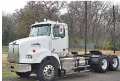
2011 Western Star 4900, D13 Detroit Engine 450 hp; 375 mi; Diesel; 10 Spd OD; Engine Brake; Air Ride; 3.55 Ratio; 24.5 Tires; Alum/Steel Wheels; 200" WB; 14,700 lb Front Axle Wt; 40,000 lb Rear Axle Wt, New. (BPBD9800-BRY-2)
