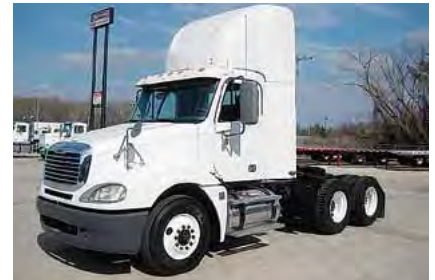
2005 Freightliner CL12064S Columbia 120 , 14.0L Detroit Engine 455 hp; 10 Spd OD; Diesel; 4 Bag Air Ride Suspension; 3.70 Ratio; 22.5LP Tires; All Steel Wheels; 171 in Wheelbase; Tandem Axle, 552,312 Miles. (5LN76723-TYL-3)
