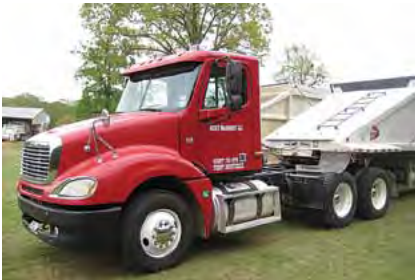
2003 Freightliner CL120 Tractor , Detroit Diesel DDC 12.7, 430 HP, 10 Spd, Air Ride Suspension, 171" Wheelbase, Steel Wheels, 22.5 LP Tires, 517,321 Miles. (3LK55310-TXK-3)
