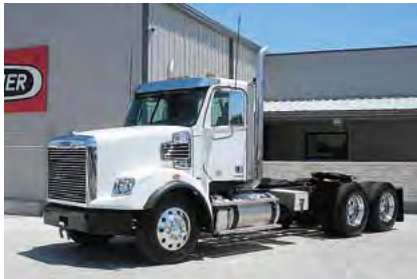
2012 Freightliner CC12264 Coronado SD , DD 15 Detroit Engine 505 hp; Diesel; 10 Spd OD; Engine Brake; Air Ride; 3.55 Ratio; 11R 24.5 Tires; Aluminum/Steel Wheels; 215 in Wheelbase; Tandem Axle, New. (CDBH0749-WAC-3)
