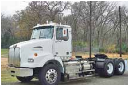
2011 Western Star 4900SA, DD 13 Detroit Engine 450 hp; 10 Spd OD; Diesel; Engine Brake; Air Ride Suspension; 3.55 Ratio; 11R 24.5 Tires; Aluminum/Steel Wheels; 200 in Wheelbase; Tandem Axle. (BDBD9799-WAC-3)
