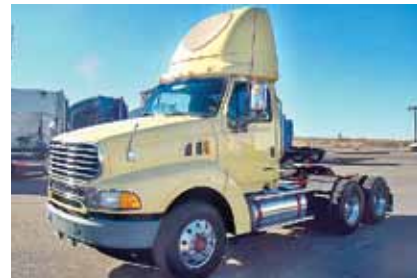
2004 Sterling AT9500, MBE4000 Mercedes Engine 410 hp; 10 Spd OD; Diesel; Engine Brake; Air Ride; 3.90 Ratio; 22.5 Tires; All Aluminum Wheels; 180" WB; Tandem Axle; 445,490 Miles. (4AM18601-ABQ-2) $28,275
