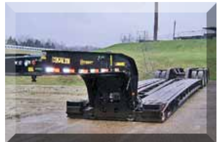
2006 Kalyn Lowboy 48'x102" AirRide, Apitong Floor, 53'x102" 25' well, 136" neck, 22' Loaded deck ht outriggers, D-rings for stinger/flip Rear axle lift, 22.5 tires Alum outsiders, Raise/lower valve, Digital Air Scale (61002469-TYL-TRL-1A) $55,000
