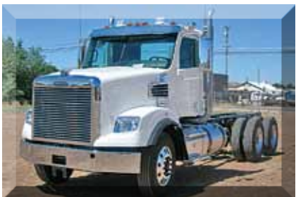
2011 Freightliner Coronado , Detroit Diesel DD15, 475 HP, 10 SPD, Engine Brake, Tuff Trac Suspension, 227 Wheelbase, Air Brakes, Tire Size 24.5, Dual Locking Differentials, Aluminum Outers, Zero Miles. (BDAW9999-FAR-1) $119,500
