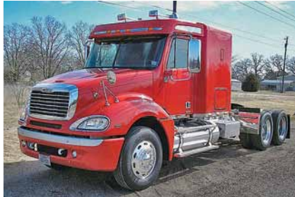
2007 Freightliner CL12064ST Columbia 120, 70 in Mid Roof XT Sleeper; 4000 Mercedes Engine 450 hp; Diesel; Automatic OD; Engine Brake; Air Ride; 3:55; 11R 24.5 Tires; Alum. Wheels; 230" WB; 250,000 Miles. (7DY74142-TEM-3)
