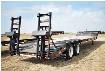
2011 Viking Tandem & Triple Axle, Fixed Neck; 45' Length, 102" Wide, Spring Susp; Wood Floor; Steel Wheels; Fixed Tandem Axle; Steel Composition; 35 Ton, 100,000# Capacity Equip. Trailer, Dove Tail & Ramps. (BN062662-SAN-TRL-3)
