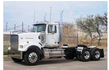
2011 Western Star 4900FA -Detroit Diesel DD15, 505 HP, 10 Spd., Engine Brake, Air Ride Suspension, 220" Wheelbase, 14K Front Axle, 40K Rear Axle, 24.5 Tires, All Aluminum Wheels, Air Brakes. New. (BPBD9615-WFF-2)
