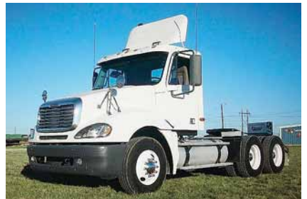
2004 Freightliner CL12064ST Columbia 120, SERIES 60 Detroit 470 hp; 10 Spd OD; Diesel; Engine Brake; Air Ride; 3.70 Ratio; 22.5 TALL Tires; All Steel Wheels; 171 in Wheelbase; Tandem Axle, 581,000 Miles. (4LM099963-SAN-2)
