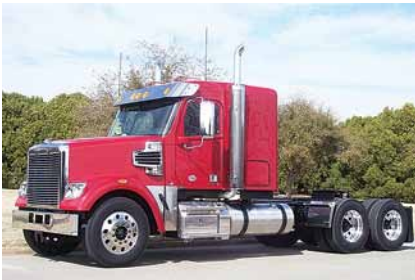
2012 Freightliner Coronado SD, 48" Mid Roof Sleeper, Detroit Diesel DD15, 505 HP, 10 Spd., Engine Brake, Air Ride Suspension, 235" Wheel Base, Dual Exhaust, 24.5 Tires, All Aluminum Wheels, New. (CDBE0093-WFF-3)
