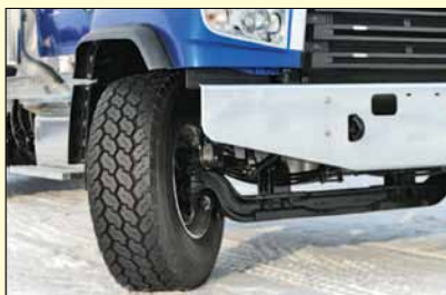
Up to 45 degree wheel cut, depending on wheel equipment.
