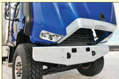
Tilt hood with radiator-mounted stationary grille and bridge formula front bumper.
