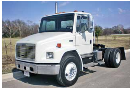
2001 Freightliner FL70, Cummins ISC, 260 HP, Allison Automatic Transmission, 12K Front Axle, 22K Rear Axle, Spring Suspension, 150" Wheelbase, 22.5 LP Tires, Steel Wheels. Single Axle Tractor. 83,000 Miles. (1HF65398-BRY-2)
