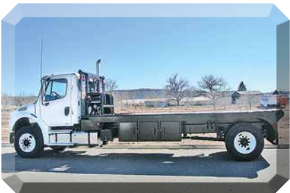
2009 Freightliner M2 106, Cab Chassis, Cummins ISC, 300 HP, 10 Speed, Engine Brake, Spring Susp, 254" WB, Roustabout Bed with Winch, Poles and Tailroller, 22.5 Tires, Steel Wheels, Air Brakes, Zero Miles. (9HAH8898-FAR-1) $107,500 $98,400
